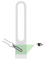
Ensure the appliance is unplugged. Look for blockages in the air inlet holes on the filter. Use a soft brush to remove debris.
