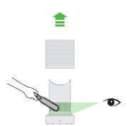
Look for blockages in the air inlet holes under the filter and use a soft brush to remove debris. Replace the filter and then the loop amplifier.
