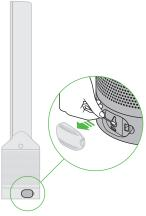
Clean the hatch every time the filter is replaced. Open the small hatch on the side of the appliance. Use a cotton bud to clean inside and remove any debris. This maintains sensor accuracy and ensures the continuing high performance of the appliance.
