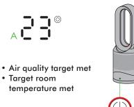
When auto mode is used while in heating mode, the appliance is both purifying and heating the air. The appliance will display the target room temperature, not the fan airflow. Once the target room temperature has been reached, the appliance will stop heating the air. If the air quality target has not been met, the fan will continue to run in order to keep purifying the air. If the room temperature falls below the target temperature, the appliance will start to heat again.
