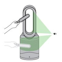
Ensure the appliance is unplugged. If the appliance has been in use, leave for 1 to 2 hours in order to allow the appliance to cool down completely. Look for blockages in the air inlet holes and in the small aperture inside the air loop amplifier. Use a soft brush to remove debris.
