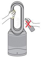
Unplug from the mains electricity supply. If the appliance has been in use, leave for 1 to 2 hours before cleaning to allow the appliance to cool completely. Dust may accumulate on the surface of the machine. Wipe dust from the loop, filter unit and other parts with a dry or damp cloth when dust accumulates. Do not use detergents or polishes.
