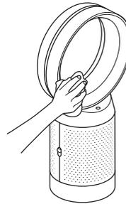
Look for blockages in the air inlet holes on the filter and the small aperture inside the loop amplifier.
