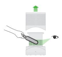
Look for blockages in the air inlet holes under the filter and use a soft brush to remove debris. Replace the filter and then the loop amplifier.
