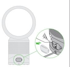
Clean the hatch every time the filter is replaced. Open the small hatch on the side of the appliance. Use a cotton bud to clean inside and remove any debris. This maintains sensor accuracy and ensures the continuing high performance of the appliance.
